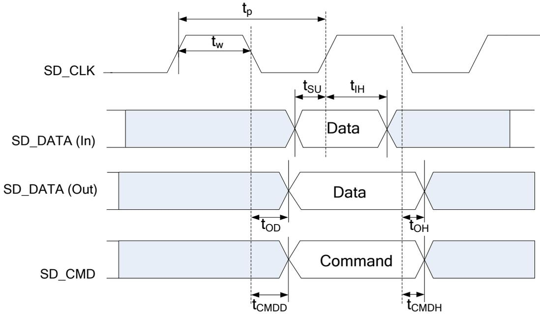
Figure 9-5 SDIO Interface Normal Timing
