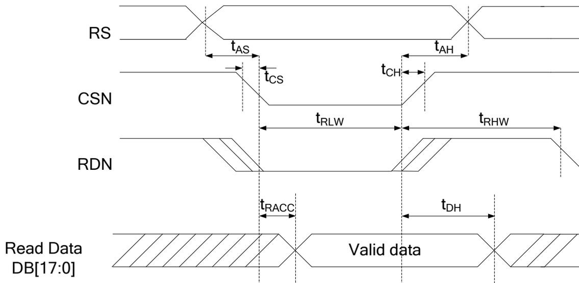
Figure 9-17 LCD Interface Timing for DBI Panel (Read Operation)
