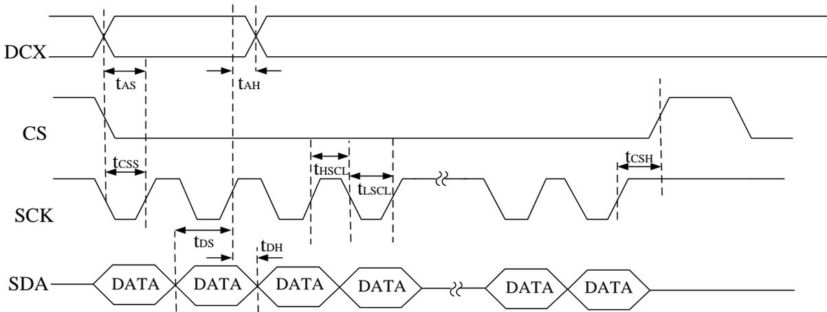
Figure 9-13 LCD Serial Interface Timing
