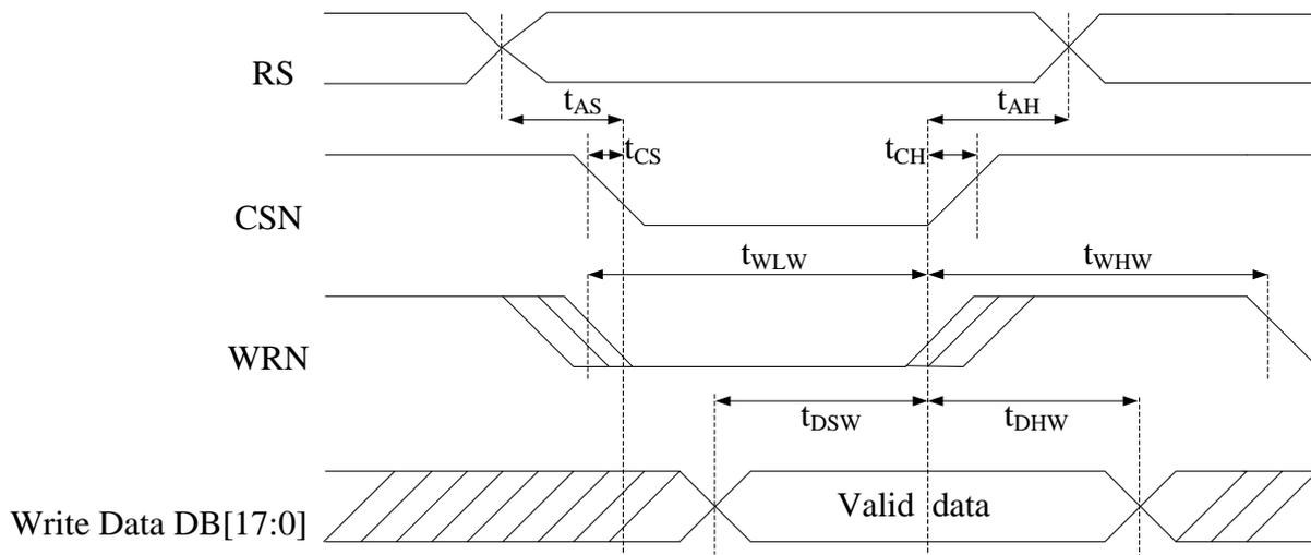
Figure 9-16 LCD Interface Timing for DBI Panel (Write Operation)
