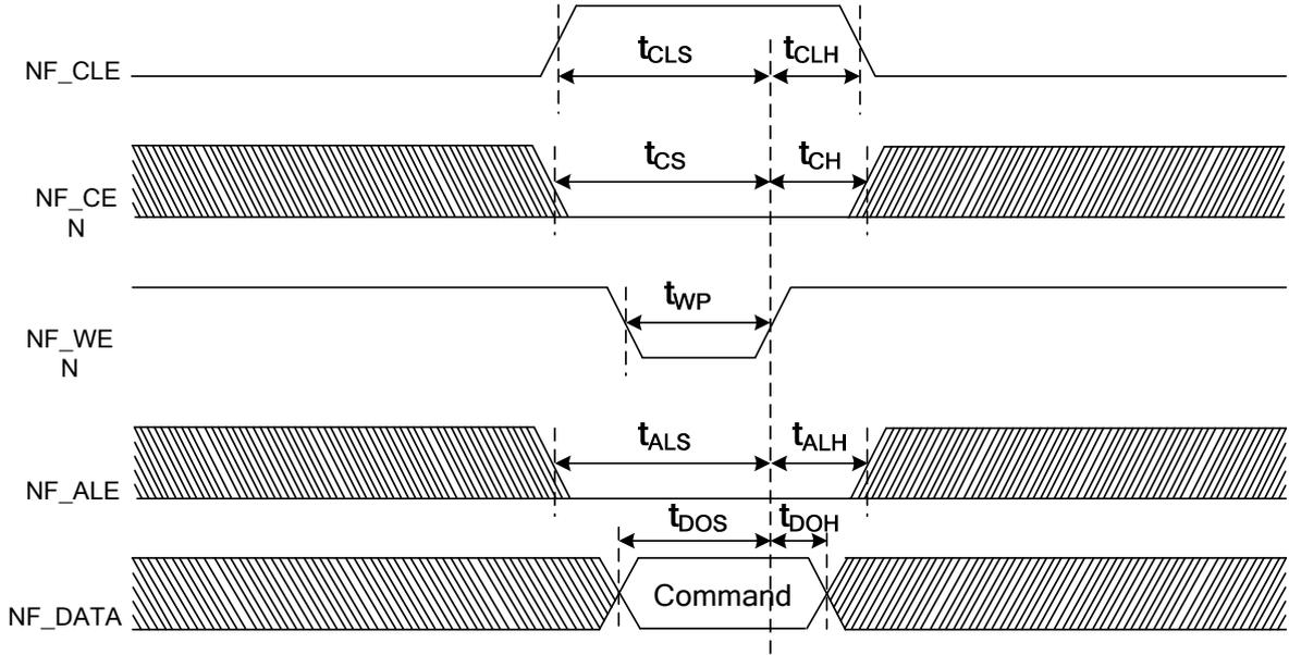
Figure 9-7 NFC Command Latch Timing
