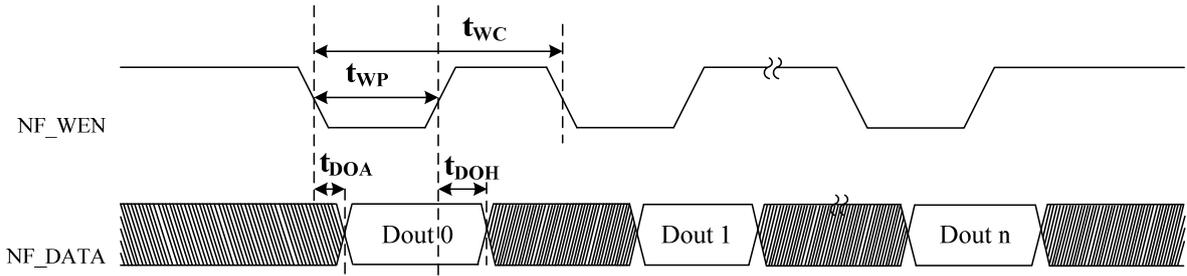
Figure 9-9 NFC Data Output Timing
