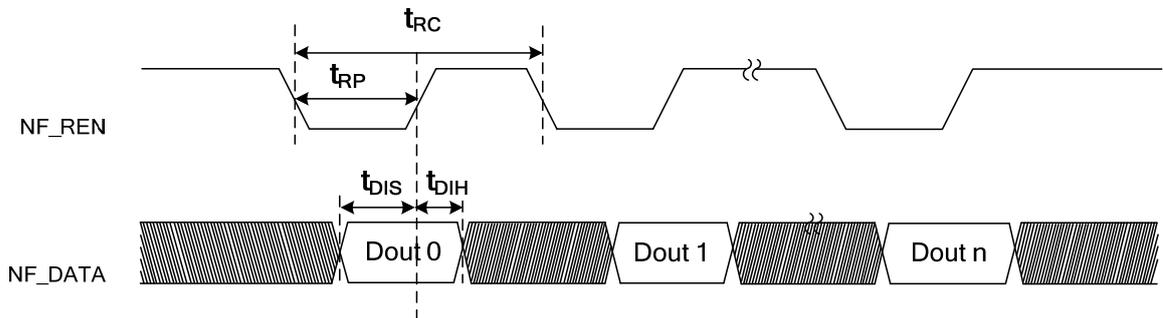
Figure 9-10 NFC Standard Data Input Timing
