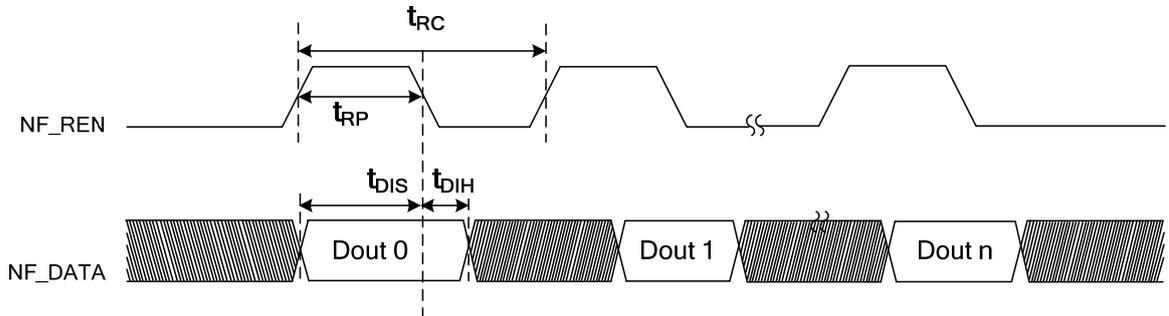
Figure 9-11 NFC EDO Data Input Timing
