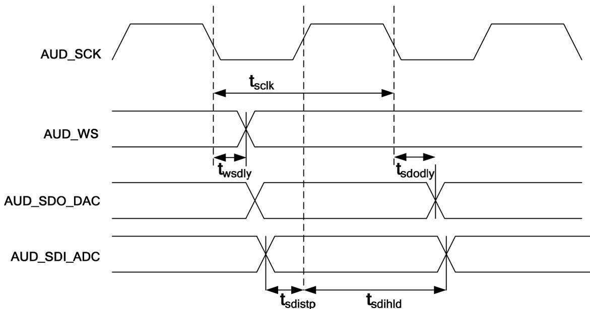
Figure 9-12 Timing Specification of I2S/PCM Serial Interface to External Devices
