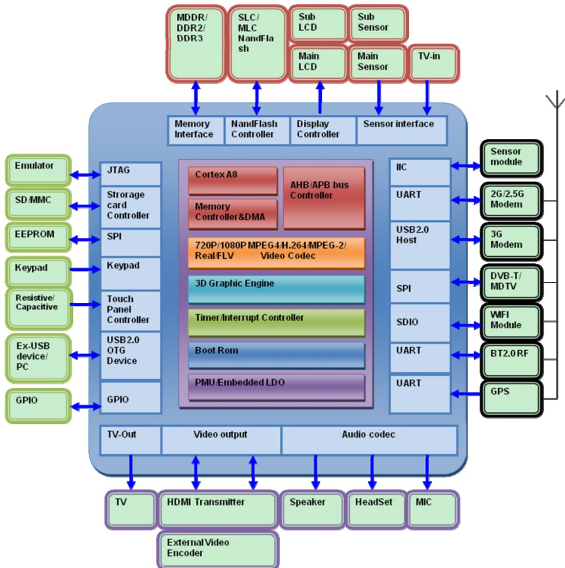
Figure 2-1 System Diagram of 445BGA
