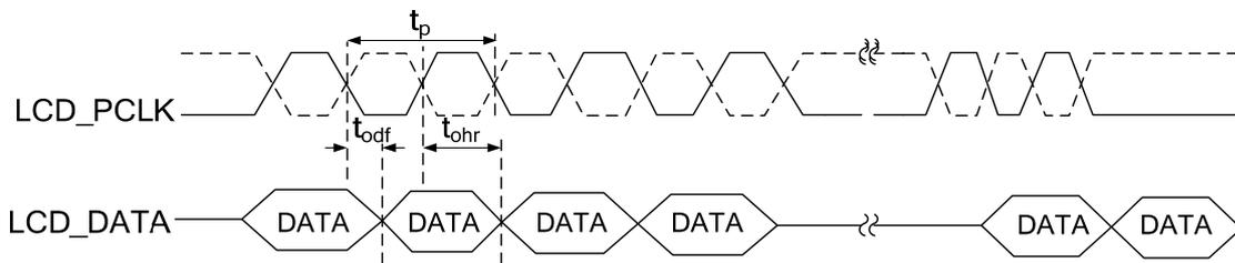
Figure 9-15 Data Output Timing for DPI Panel (rising edge capture)
