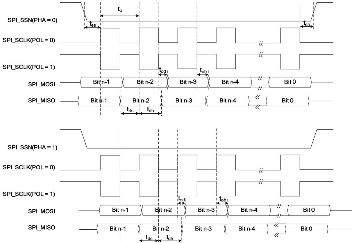
Figure 9-3 SPI Interface--Transmit and Receive in Master Mode
