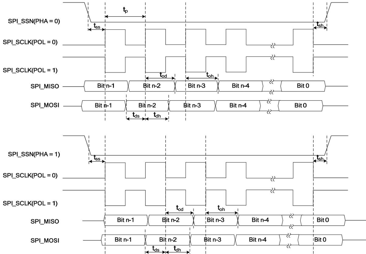
Figure 9-2 SPI Interface--Transmit and Receive in Slave Mode
