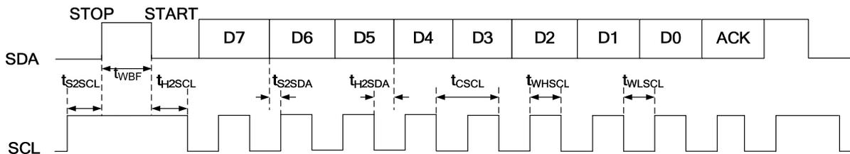
**Figure 9-4 I2C Interface Timing**
