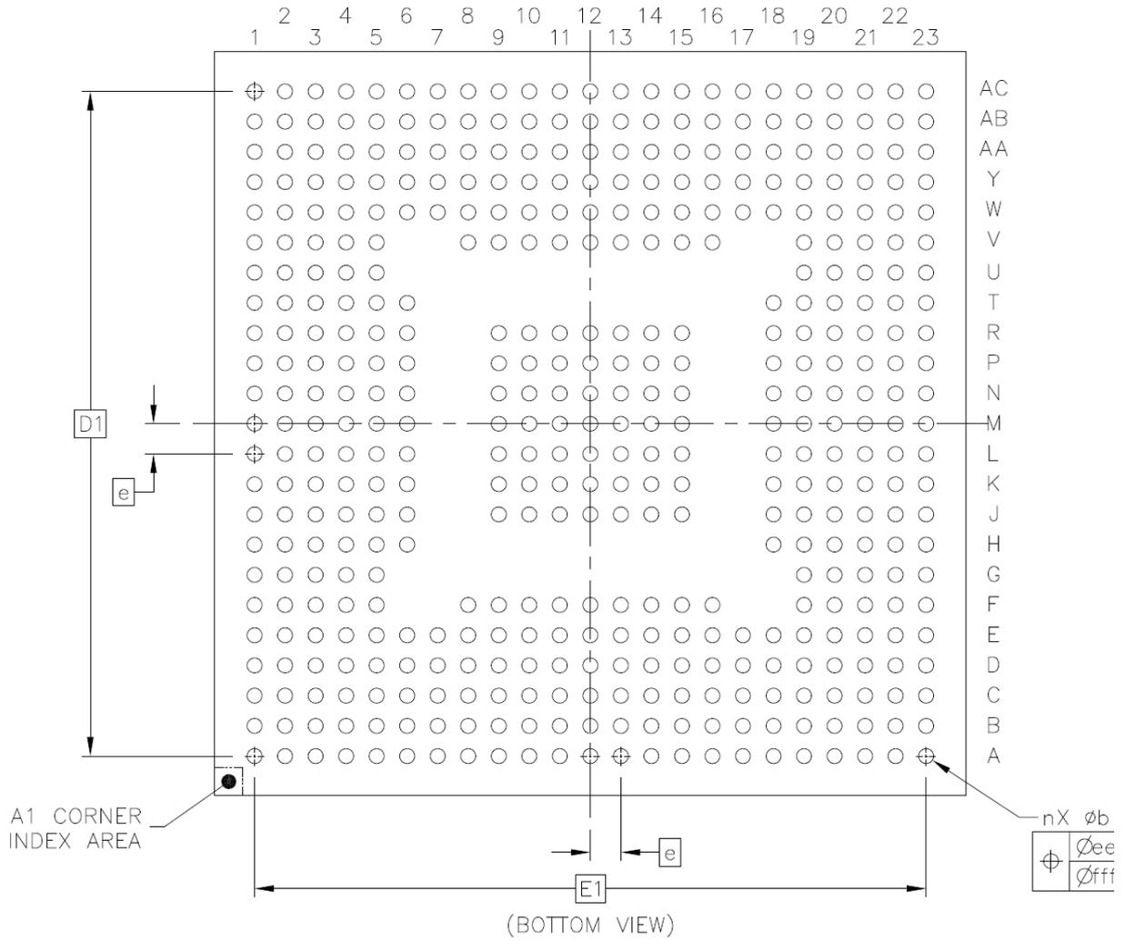
Figure 3-6 Bottom View of 445BGA Package
