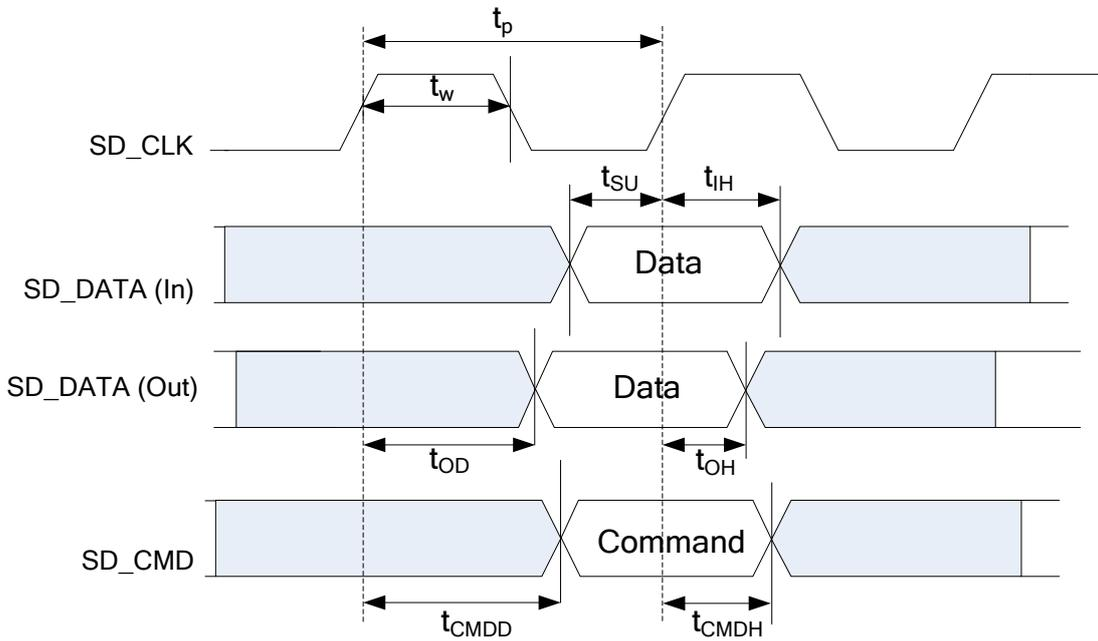
Figure 9-6 SDIO Interface High Speed Timing
