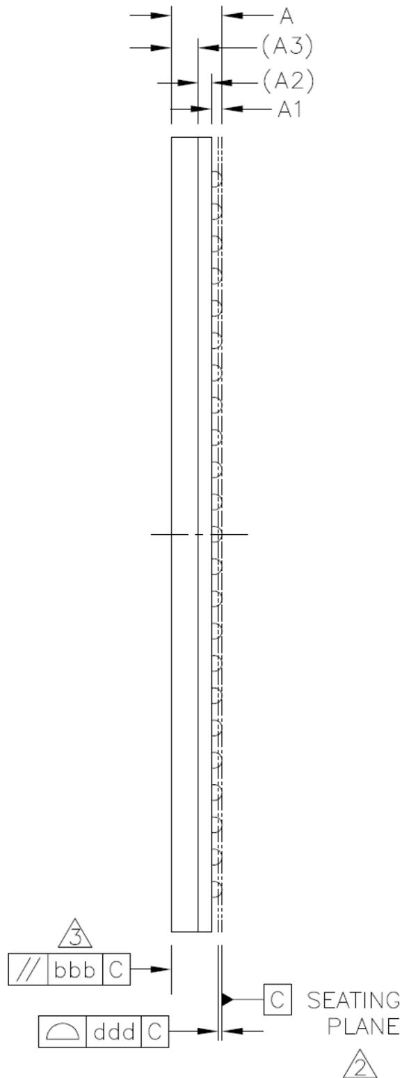
**Figure 3-7 Side View of 445BGA Package**
