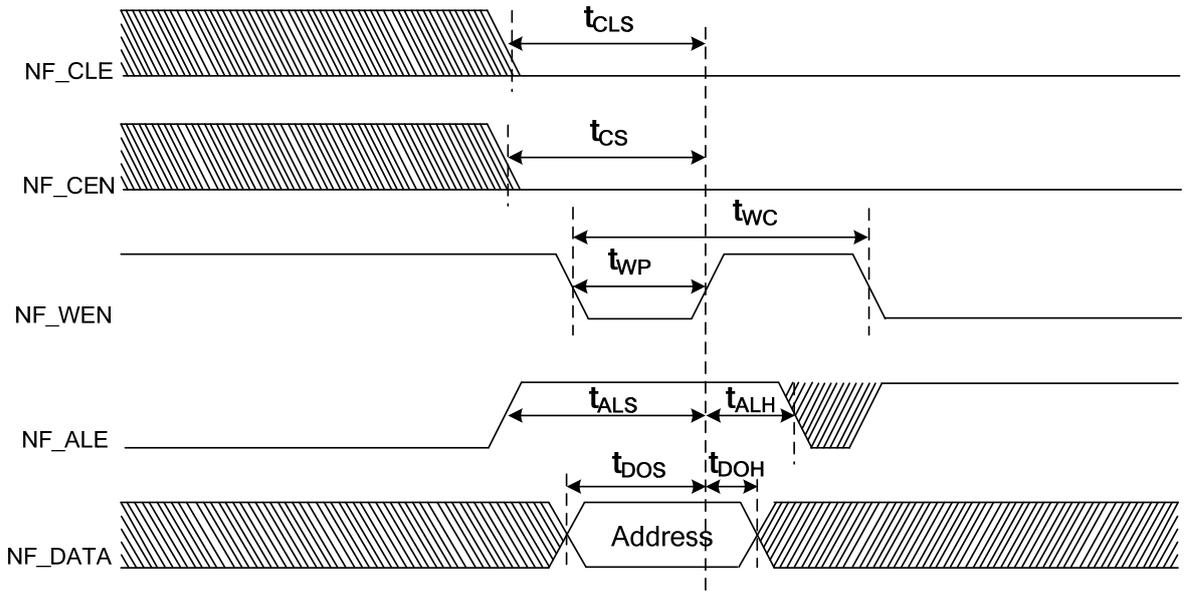
Figure 9-8 NFC Address Latch Timing
