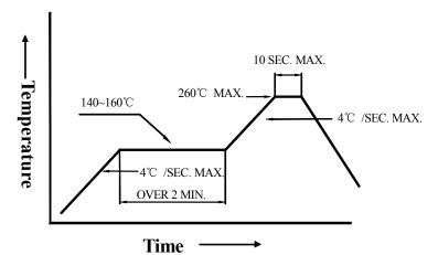
3). DIP soldering (Wave Soldering):
