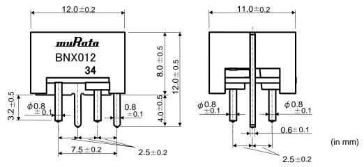
( The tip by solder of terminal is not included in the dimension values. )
