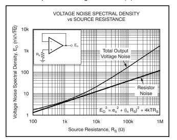
Figure 31. Noise Performance of the OPA1611 in Unity-Gain Buffer Configuration
