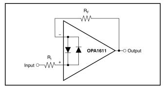
Figure 30. Pulsed Operation
