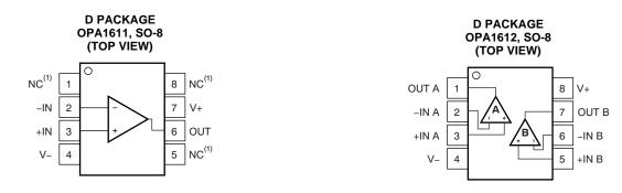
(1) NC denotes no internal connection. Pin can be left floating or connected to any voltage between (V-) and (V+).
