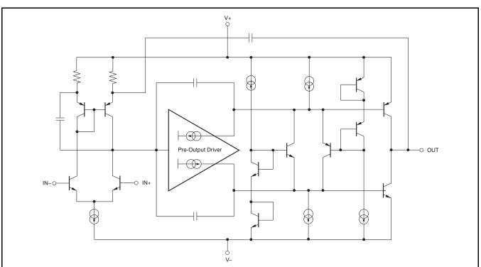
Figure 29. OPA1611 Simplified Schematic
