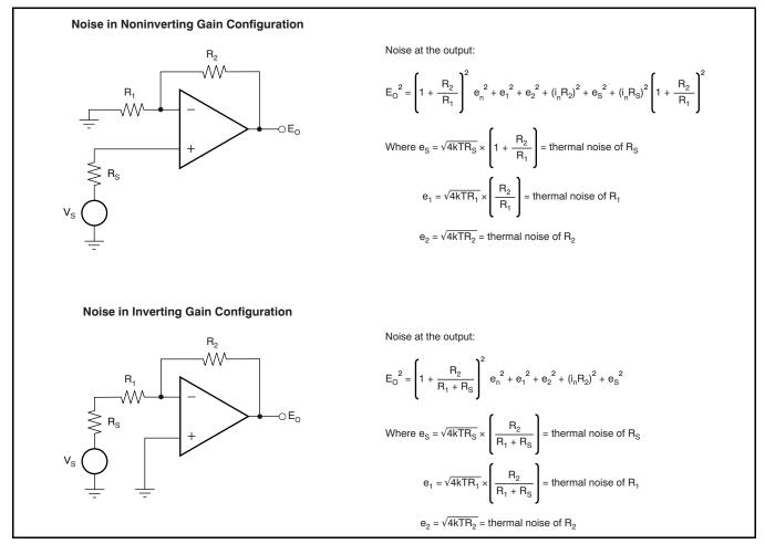
For the OPA161x series op amps at 1kHz,  $e_n$  = 1.1nV/ $\sqrt{Hz}$  and  $i_n$  = 1.7pA/ $\sqrt{Hz}.$
