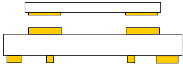
Figure 21. Correct PCB Top Metal Pattern Under Package
