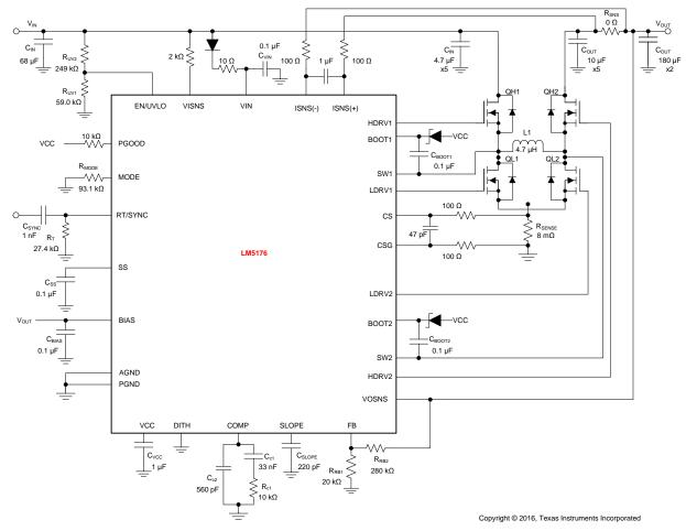
Figure 25. LM5176 Four-Switch Buck Boost Application Schematic
