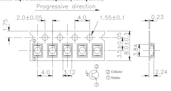
TOLERANCES UNLESS DIMENSION±0.1 ANGLE±0.5 UNIT:mm
