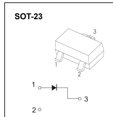
Solid dot = Green molding compound device, if none, the normal device.
