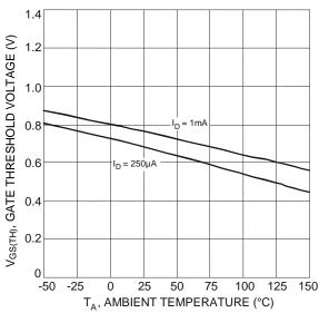
Fig. 7 Gate Threshold Variation vs. Ambient Temperature
