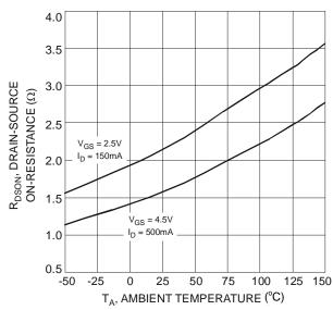
Fig. 6 On-Resistance Variation with Temperature
