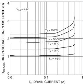
Fig. 4 Typical On-Resistance vs. Drain Current and Temperature
