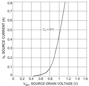
Fig. 8 Diode Forward Voltage vs. Current
