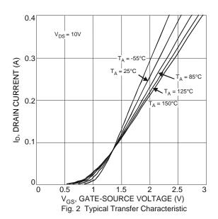
Short duration pulse test used to minimize self-heating effect.
