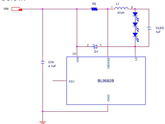
A value of 1µF will reduce the supply ripple current by a factor three (approx.). Proportionally lower ripple can be achieved with higher capacitor values. Note that the capacitor will not affect operating frequency or efficiency, but it will increase start-up delay and reduce the frequency of
