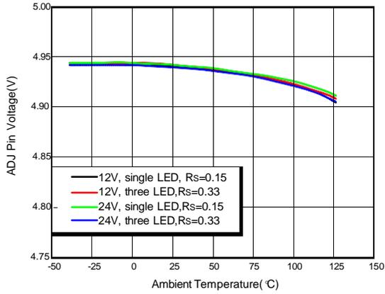
**Voltage across R<sub>SENSE</sub> Vs. Temperature**
