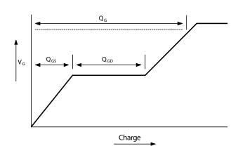
Basic gate charge waveform
