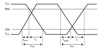
Switching time waveforms
