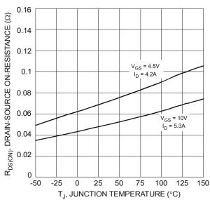
Figure 6 On-Resistance Variation with Temperature
