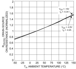
Figure 5 On-Resistance Variation with Temperature
