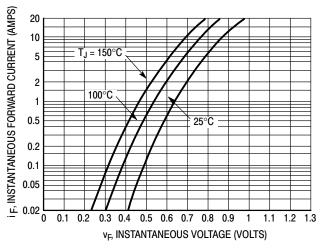
Figure 1. Typical Forward Voltage
