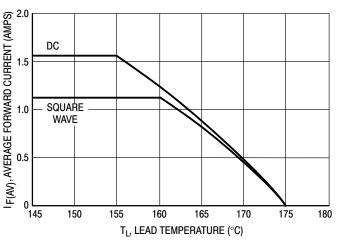
Figure 4. Current Derating, Lead
