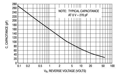
Figure 5. Typical Capacitance
