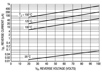
Figure 2. Typical Reverse Current\*
