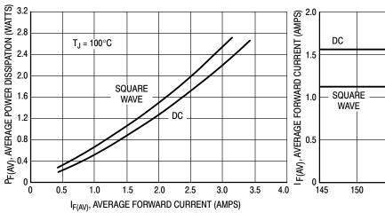
Figure 3. Power Dissipation
