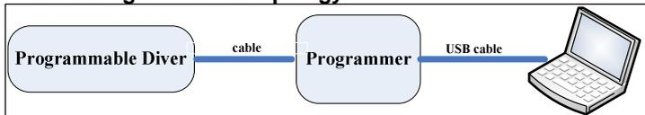
The programmable driver can be programmed by using special PC software and the programmer module.
