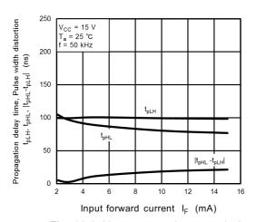
Fig. 12.2.19  $t_{pHL}, t_{pLH}, |t_{pHL}-t_{pLH}| - I_F$
