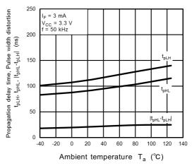
Fig. 12.2.14  $t_{pHL}, t_{pLH}, |t_{pHL}-t_{pLH}| - T_a$
