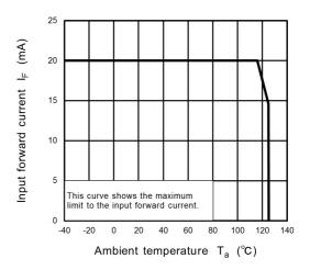
Fig. 12.2.2 I<sub>F</sub> - T<sub>a</sub>
