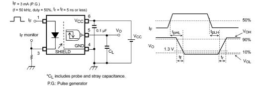
Fig. 12.1.7 Switching Time Test Circuit and Waveform
