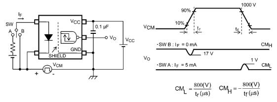
Fig. 12.1.8 Common-Mode Transient Immunity Test Circuit and Waveform
