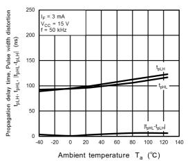
Fig. 12.2.16 t<sub>pHL</sub>,t<sub>pLH</sub>,|t<sub>pHL</sub>-t<sub>pLH</sub>| - T<sub>a</sub>
