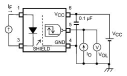
Fig. 12.1.1 V<sub>OL</sub> Test Circuit
