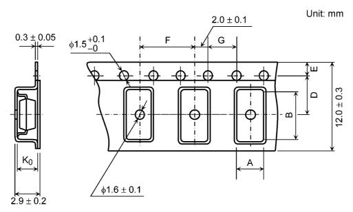
Table Tape Dimensions (unit: mm, tolerance: ±0.1)
