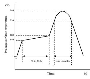
This profile is based on the devices maximum heat resistance guaranteed value. Set the preheat temperature/heating temperature to the optimum temperature corresponding to the solder paste type used by the customer within the described profile.
