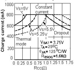
Fig.4:The relationship curve between charge current with Rcc
