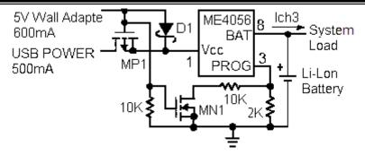
Fig.5:Combining Wall Adapter and USB Power
