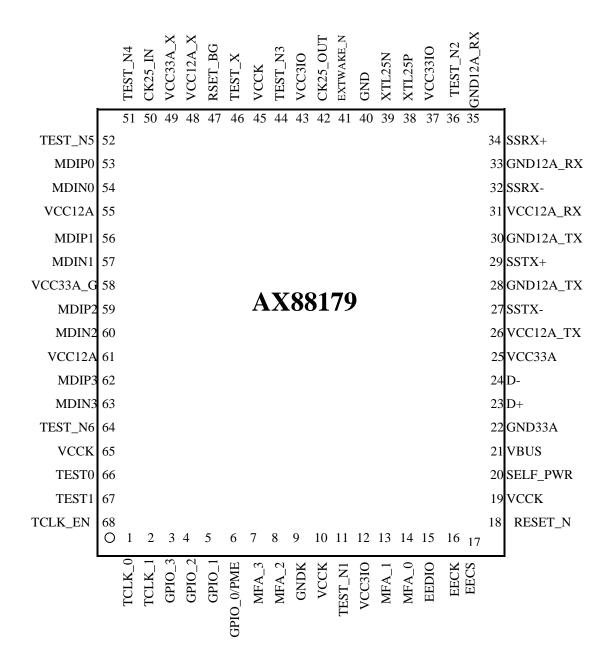
Figure 3 : Pinout Diagram
