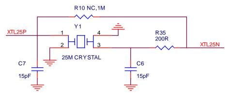
Figure 4 : 25MHz Crystal Reference Circuit
