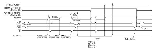
**Note:** The wave-form chart is based on the case of 7 data bit length + parity bit + 2 stop bit.
