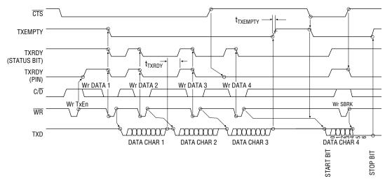
**Note:** The wave-form chart is based on the case of 7-bit data length + parity bit + 2 stop bit.
