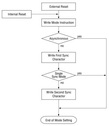
Fig. 1 Function-setting Sequence (Mode Instruction Sequence)
