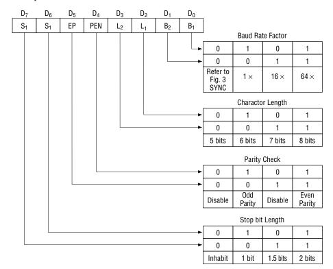
Fig. 2 Bit Configuration of Mode Instruction (Asynchronous)
