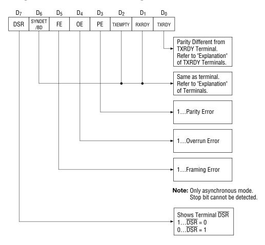
Fig. 5 Bit Configuration of Status Word
