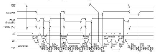
Note: The wave-form chart is based on the case of 5 data bit length + parity bit and 2 synchronous charactors.
