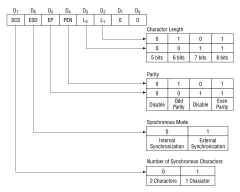
Fig. 3 Bit Configuration of Mode Instruction (Synchronous)
