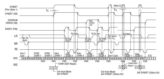
Note: 1. Internal Synchronization is based on the case of 5 data bit length + parity bit and 2 synchronous charactor.
