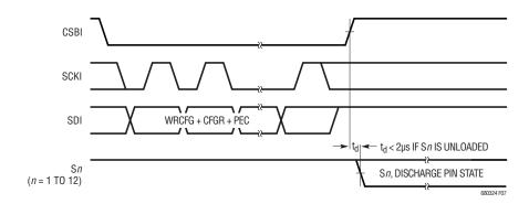
Figure 7. S Pin Action and SPI Transmission
