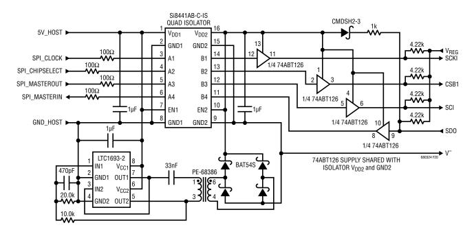
Figure 20. Providing an Isolated High Speed Data Interface
