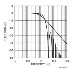
Figure 25. Noise Filtering of the LTC6803-4 ADC
