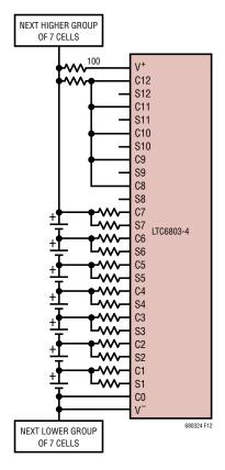
Figure 12. Monitoring 7 Cells with the LTC6803-4
