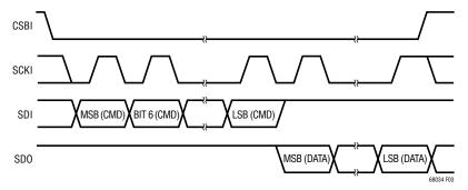
Figure 3. Transmission Format (Read)
