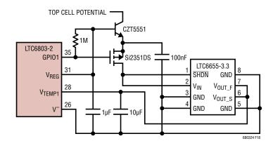
Figure 18. Providing Measurement of Calibration Reference
