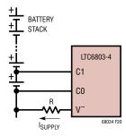
Figure 22. Kelvin Connection on CO Improving Bottom Cell Voltage Measurement Accuracy
