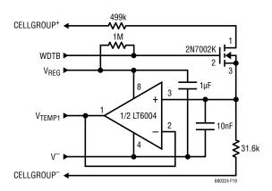
Figure 19. Using a V<sub>TEMP</sub> Input for Full-Stack Readings
