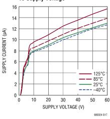
Supply Current vs Supply Voltage During Continuous Conversions
