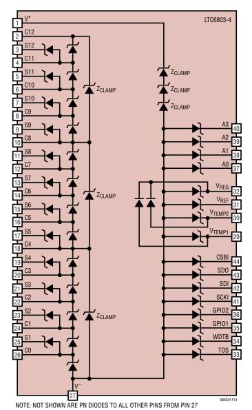
Figure 13. Internal Protection Diodes
