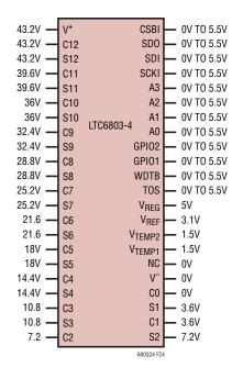
Figure 24. Typical Pin Voltages for Twelve 3.6V Cells
