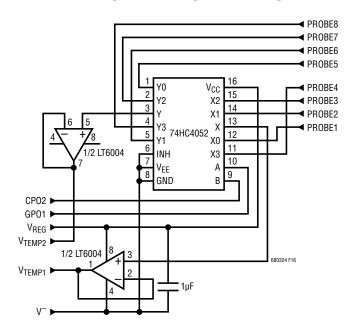
Figure 16. Expanding Sensor Count with Multiplexing
