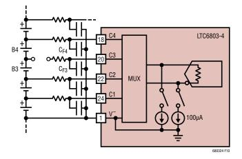
Figure 10. Open Connection with RC Filtering
