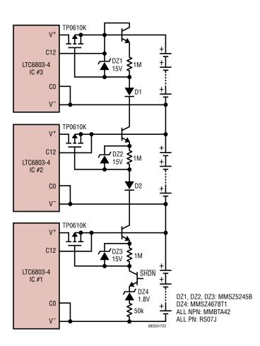
Figure 23. Hardware Shutdown Circuit Reduces Total Supply Current of LTC6803-4 to About OµA
