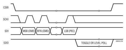
Figure 6. Transmission Format (PLADC Conversion or PLINT)
