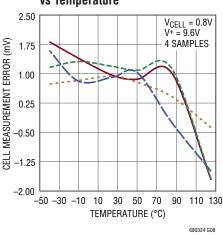
Cell 3 to Cell 12 Voltage Measurement Error vs Temperature
