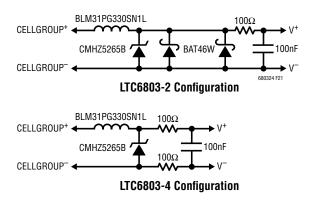
Figure 21. Supply Decoupling
