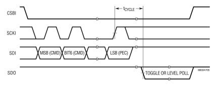
Figure 5. Transmission Format (ADC Conversion and Poll)
