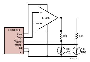
Figure 15. Buffering V<sub>REF</sub> for Higher Current Sensors
