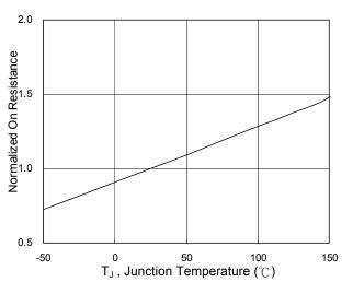
Fig.6 Normalized R<sub>DSON</sub> vs. T<sub>J</sub>
