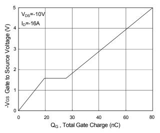
Fig.4 Gate-Charge Characteristics
