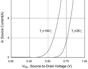
Fig.3 Forward Characteristics of Reverse
