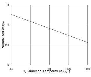
Fig.5 Normalized  $V_{GS(th)}$  vs.  $T_J$
