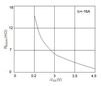
Fig.2 On-Resistance vs. G-S Voltage
