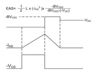
Fig.11 Unclamped Inductive Switching Waveform
