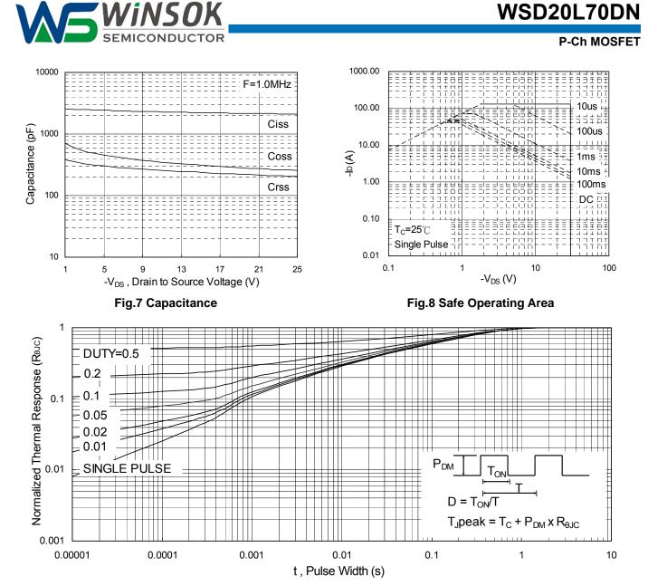
Fig.9 Normalized Maximum Transient Thermal Impedance
