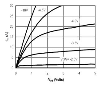
Figure 2. Drain Current
