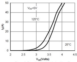
Figure 2: Transfer Characteristics (Note E)
