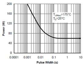
Figure 10: Single Pulse Power Rating Junction-to-Case (Note F)
