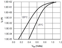
Figure 6: Body-Diode Characteristics (Note E)
