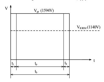
$$\begin{array}{lll} t_3, & t_4 & = 0.1 \text{ s} \\ t_p & \text{(Partial discharge measuring time)} & = 1 \text{ s} \\ t_b & = 1.2 \text{ s} \end{array}$$
