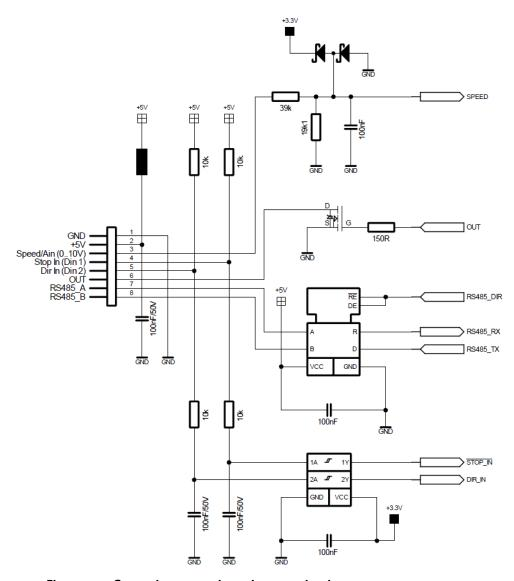
Figure 4.5: General purpose input/output circuit
