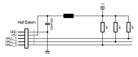
Figure 4.3: Hall sensor input circuit
