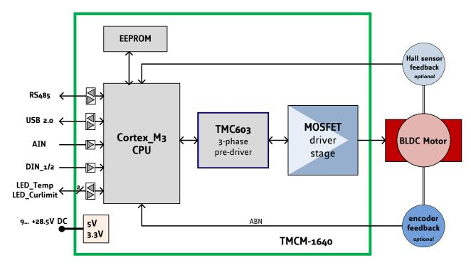
Figure 6.1: Main parts of the TMCM-1640
