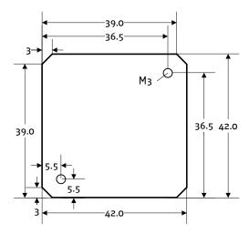
Figure 4.1: Module dimension and position of mounting holes
