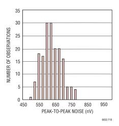
Figure 18. LTC6655-2.5 Low Frequency Noise Histogram
