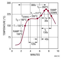
Figure 24. Lead-Free Reflow Profile
