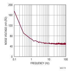
Figure 19. LTC6655-2.5 Low Frequency Noise Spectrum
