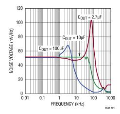
Figure 1. Output Voltage Noise Spectrum
