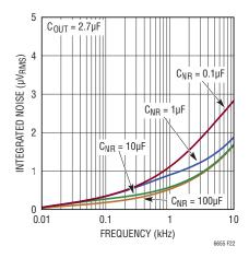
Figure 22. Total Integrated Noise of the LTC6655LN-2.5 Using the C<sub>NR</sub> Capacitor
