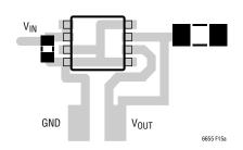
Figure 15a. Sample LTC6655 PCB Layout
