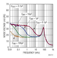
Figure 21. The LTC6655LN-2.5 Output Voltage Noise Spectrum Using the C<sub>NR</sub> Capacitor
