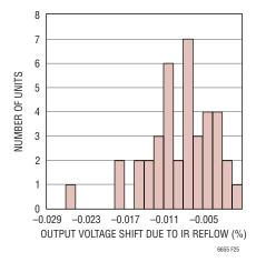
Figure 25. Output Voltage Shift Due to IR Reflow
