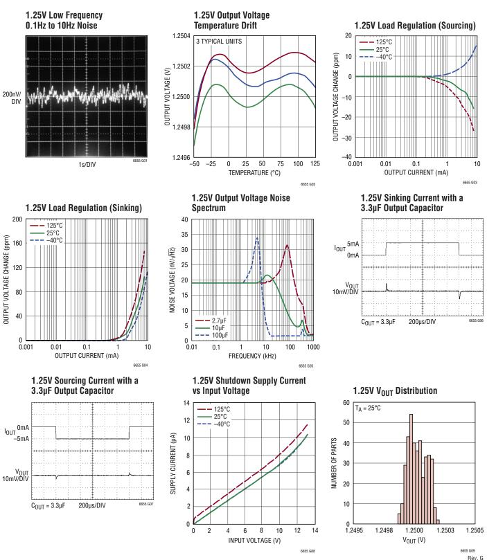
Characteristic curves are similar for most voltage options of the LTC6655. Curves from the LTC6655-1.25, LTC6655-2.5 and the LTC6655-5 represent the range of performance across the entire family of references. Characteristic curves for other output voltages fall between these curves and can be estimated based on their voltage output.
