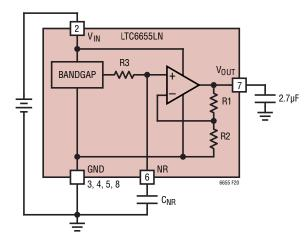
Figure 20. The LTC6655LN Typical Application Circuit
