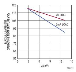
Figure 14. LTC6655-2.5 Maximum Ambient Operating Temperature
