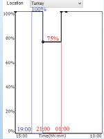
For above figure, the driver will output 75% for 4hours, after it outputs 100% for 2hours.
