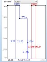
For above figure, the driver will output 100% for 2hours, after it outputs 100% for 2hours, outputs 75% for 4hours, outputs 30% for 2hours
