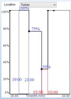
For above figure, the driver will output 30% for 2hours, after it outputs 100% for 2hours, outputs 75% for 4hours
