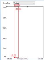
For above figure, you can regard 19:00 (starting point) as that the driver is turned on. It will keep 100% output for 2hours, so the second point should be 21:00.
