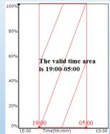
The most important point is that 19:00 is the starting point in the dimming plan, you can regard it as turn on driver.
