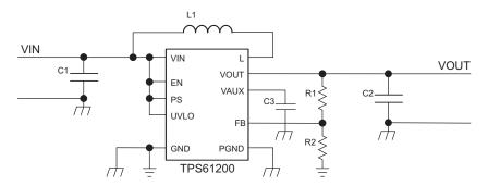
Figure 14. Parameter Measurement Schematic
