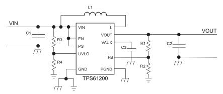
Figure 15. Typical Application Circuit for Adjustable Output Voltage Option
