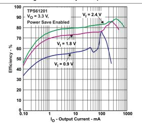
Figure 4. Efficiency vs Output Current
