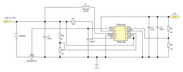
Figure 28. Reverse Battery Protection Circuit (See SLVA315)
