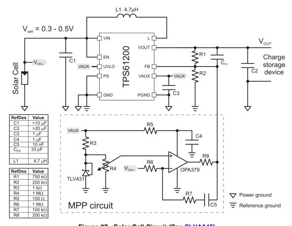
Figure 27. Solar Cell Circuit (See SLVA345)
