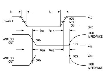
Figure 11a. Propagation Delays, Enable to Analog Out
