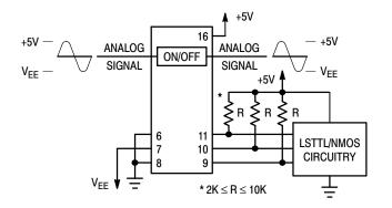
a. Using Pull-Up Resistors
