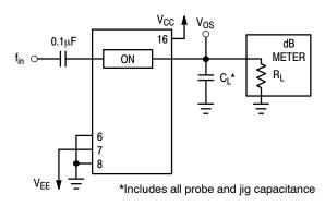
Figure 6. Maximum On Channel Bandwidth, Test Set-Up
