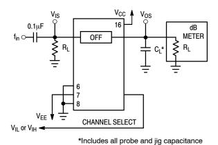
Figure 7. Off Channel Feedthrough Isolation, Test Set-Up
