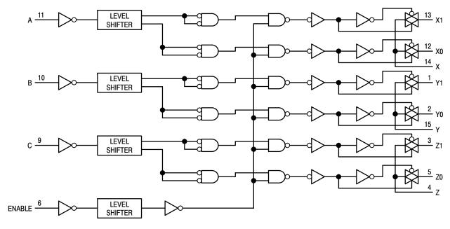
Figure 20. Function Diagram, HC4053A
