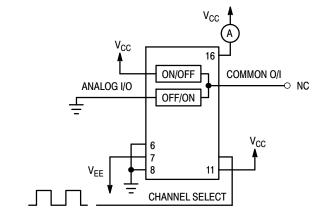
Figure 13. Power Dissipation Capacitance, Test Set-Up
