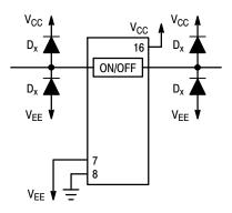
Figure 16. External Germanium or Schottky Clipping Diodes
