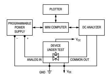
Figure 2. On Resistance Test Set-Up
