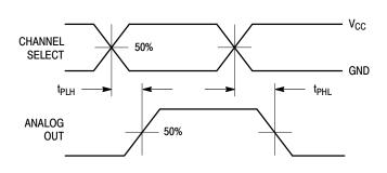
Figure 9a. Propagation Delays, Channel Select to Analog Out
