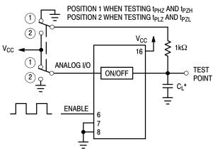
Figure 11b. Propagation Delay, Test Set-Up
