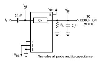
Figure 14a. Total Harmonic Distortion, Test Set-Up
