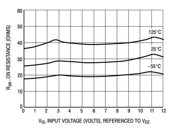
Figure 1e. Typical On Resistance,  $V_{CC}$  –  $V_{EE}$  = 9.0 V
