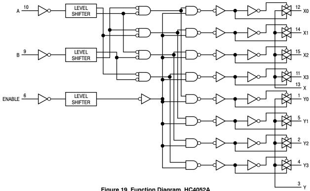
Figure 19. Function Diagram, HC4052A
