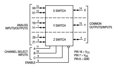
NOTE: This device allows independent control of each switch. Channel–Select Input A controls the X–Switch, Input B controls the Y–Switch and Input C controls the Z–Switch
