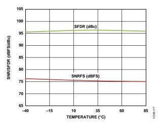
Figure 18. SNR/SFDR vs. Temperature;  $f_{IN} = 9.7$  MHz,  $f_{SAMPLE} = 65$  MSPS
