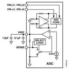
Figure 34. Internal Reference Configuration
