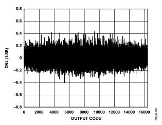
Figure 20. DNL;  $f_{IN} = 9.7$  MHz,  $f_{SAMPLE} = 65$  MSPS
