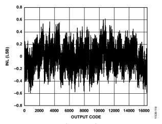
Figure 19. INL;  $f_{IN} = 9.7 \text{ MHz}$ ,  $f_{SAMPLE} = 65 \text{ MSPS}$
