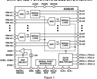
The ADC contains several features designed to maximize flexibility and minimize system cost, such as programmable clock and data alignment and programmable digital test pattern generation.
