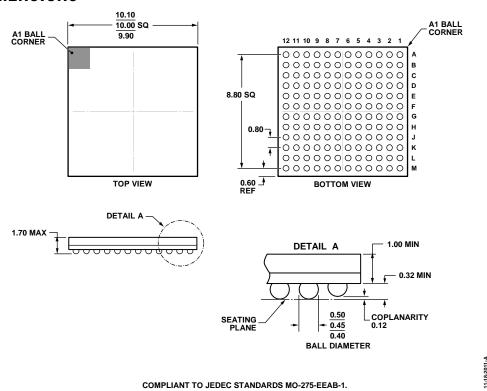
Figure 51. 144-Ball Chip Scale Package Ball Grid Array [CSP\_BGA] (BC-144-7) Dimensions shown in millimeters
