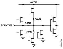
Figure 26. Equivalent SDIO/DFS Input Circuit
