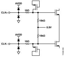
Figure 25. Equivalent Clock Input Circuit
