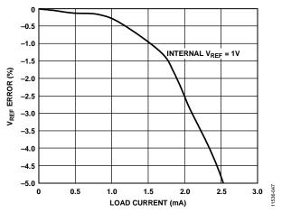
Figure 37. V<sub>REF</sub> Error vs. Load Current
