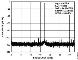
Figure 9. Single-Tone 32k FFT with  $f_{IN} = 48$  MHz,  $f_{SAMPLE} = 65$  MSPS
