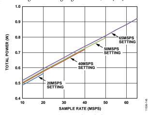
Figure 45. Total Power vs.  $f_{SAMPLE}$  for  $f_{IN} = 9.7$  MHz
