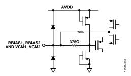
Figure 29. Equivalent RBIASx and VCMx Circuit
