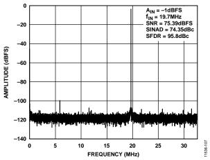
Figure 8. Single-Tone 32k FFT with  $f_{IN} = 19.7$  MHz,  $f_{SAMPLE} = 65$  MSPS
