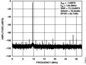
Figure 12. Single-Tone 32k FFT with  $f_{IN} = 139.5$  MHz,  $f_{SAMPLE} = 65$  MSPS
