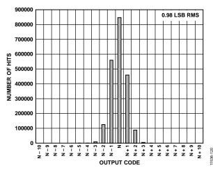
Figure 21. Input Referred Noise Histogram;  $f_{SAMPLE} = 65 \text{ MSPS}$
