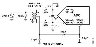
Figure 36. Differential Transformer Coupled Configuration for Baseband Applications
