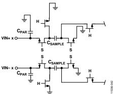
Figure 32. Switched Capacitor Input Circuit
