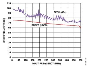
Figure 17. SNR/SFDR vs. f<sub>IN</sub>; f<sub>SAMPLE</sub> = 65 MSPS
