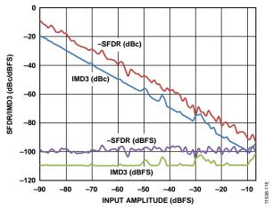
Figure 16. Two-Tone SFDR/IMD3 vs. Input Amplitude;  $f_{\rm IN1}=30.1$  MHz,  $f_{\rm IN2}=32.1$  MHz,  $f_{\rm SAMPLE}=65$  MSPS
