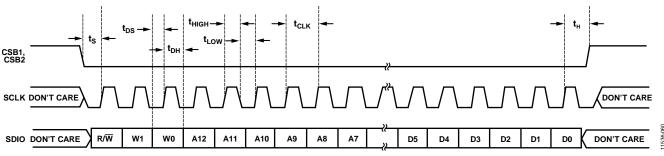
Figure 50. Serial Port Interface Timing Diagram
