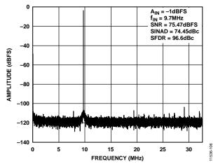
Figure 7. Single-Tone 32k FFT with  $f_{IN} = 9.7$  MHz,  $f_{SAMPLE} = 65$  MSPS
