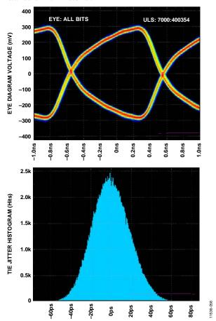
Figure 48. Data Eye for LVDS Outputs in ANSI-644 Mode with Trace Lengths of Less Than 24 Inches on Standard FR-4 Material, External 100  $\Omega$  Far End Termination Only
