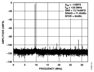
Figure 13. Single-Tone 32k FFT with  $f_{\text{IN}} = 139.5$  MHz,  $f_{\text{SAMPLE}} = 65$  MSPS, Clock Divider = 4
