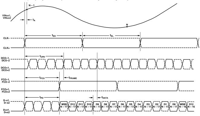
Figure 3. Wordwise DDR,  $1 \times$  Frame, 14-Bit Output Mode (Default)
