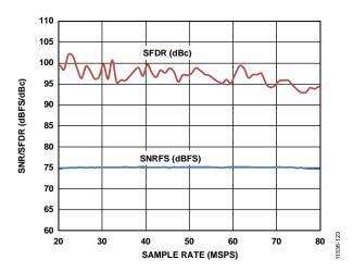
Figure 23. SNR/SFDR vs. Sample Rate;  $f_{IN} = 19.7$  MHz,  $f_{SAMPLE} = 65$  MSPS
