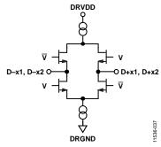
Figure 27. Equivalent Digital Output Circuit
