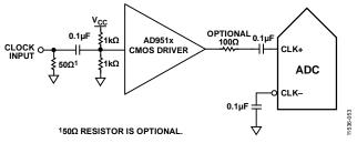
Figure 43. Single-Ended 1.8 V CMOS Input Clock (Up to 200 MHz)
