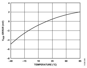
Figure 38. Typical V<sub>REF</sub> Drift
