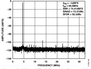
Figure 10. Single-Tone 32k FFT with  $f_{IN} = 69.5$  MHz,  $f_{SAMPLE} = 65$  MSPS
