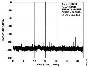
Figure 11. Single-Tone 32k FFT with  $f_{IN} = 118$  MHz,  $f_{SAMPLE} = 65$  MSPS
