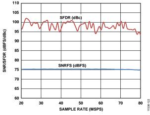
Figure 22. SNR/SFDR vs. Sample Rate;  $f_{IN} = 9.7$  MHz,  $f_{SAMPLE} = 65$  MSPS
