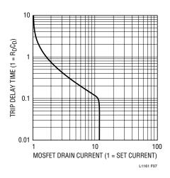
Figure 7. Current Limit Delay Time
