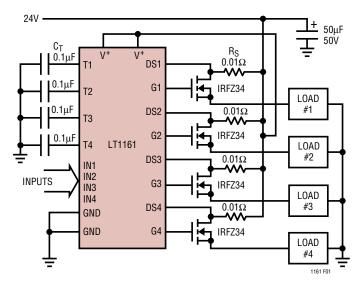
Figure 1. Protected Quad High-Side Switch
