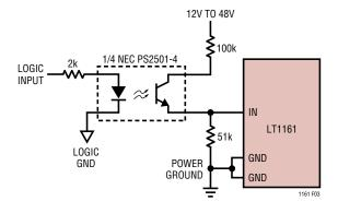
Figure 3. Isolating the Inputs
