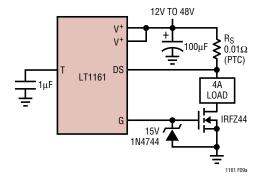
Figure 9a. Low-Side Driver with Load Current Sensing
