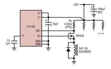
Figure 4. Drain Sense Configuration
