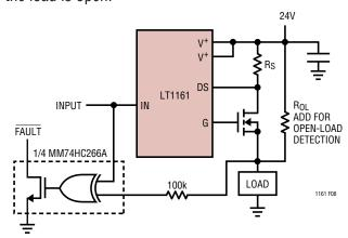
Figure 8. Fault Feedback Using Exclusive-NOR Gate
