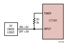
Figure 5. Latch-Off Input Network (Auto-Restart Defeated)
