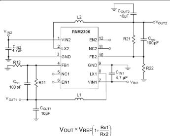
Figure 1. Adjustable Voltage Regulator
