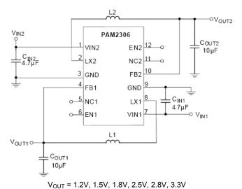
Figure 2. Fixed Voltage Regulator
