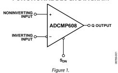
The TTL-/CMOS-compatible output stage is designed to drive up to 15 pF with full rated timing specifications and to degrade in a graceful and linear fashion as additional capacitance is added. The input stage of the comparator offers robust protection against large input overdrive, and the outputs do not phase reverse when the valid input signal range is exceeded.
