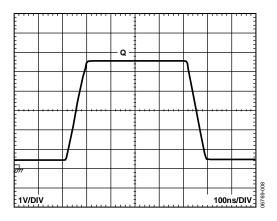
Figure 8. 1 MHz Output Voltage Waveform  $V_{CC} = 5.5 \text{ V}$
