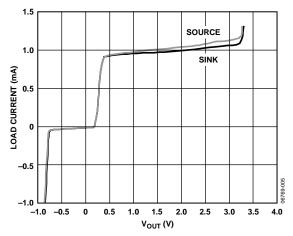
Figure 5. Load Current (mA) vs. V<sub>OH</sub>/V<sub>OL</sub>
