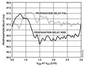
Figure 6. Propagation Delay vs. Input Common-Mode Voltage
