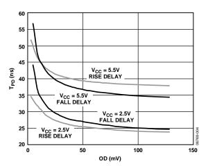
Figure 4. Propagation Delay vs. Input Overdrive at  $V_{CC} = 2.5 \text{ V}$  and 5.5 V
