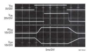
Figure 4. Start-Up Waveforms with Soft-Start Circuit Added
