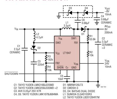
Figure 1, 3,3V Powered TFT-LCD Bias Generator
