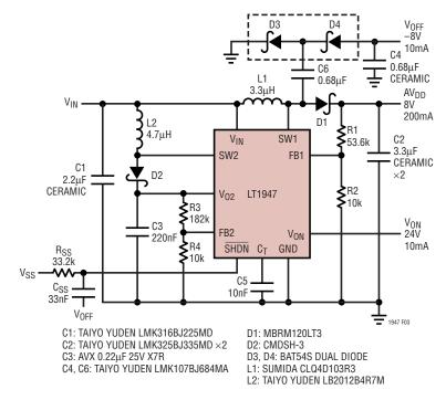
Figure 3.  $R_{SS}$  and  $C_{SS}$  at  $\overline{\mbox{SHDN}}$  Pin Provide Soft-Start
