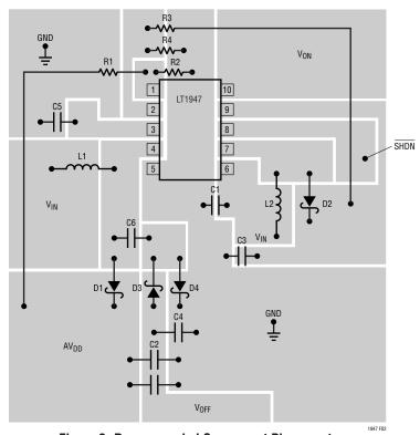
Figure 2. Recommended Component Placement
