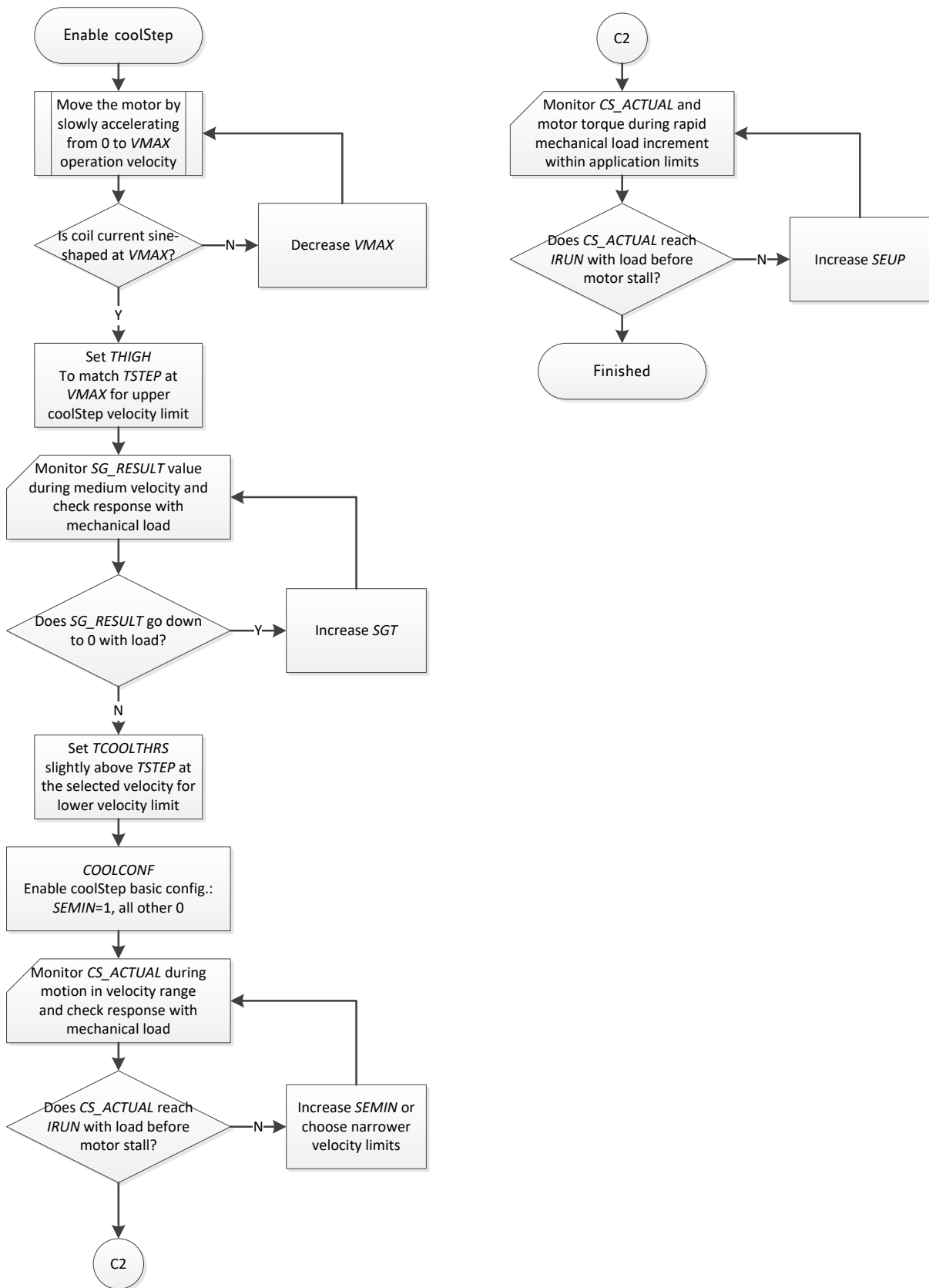
Figure 18.3 Enabling coolStep (only in combination with spreadCycle)
