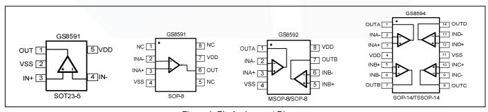
Figure 1. Pin Assignment Diagram
