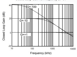
Closed Loop Gain vs. Frequency at +2.5V
