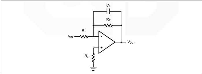
Figure 5. Low Pass Active Filter
