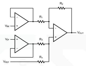
Figure 6. Instrument Amplifier
