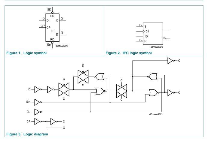
Low-power D-type flip-flop with set and reset; positive-edge trigger
