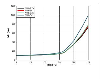
Figure 9. Supply Current vs. Temperature, Sleep Mode
