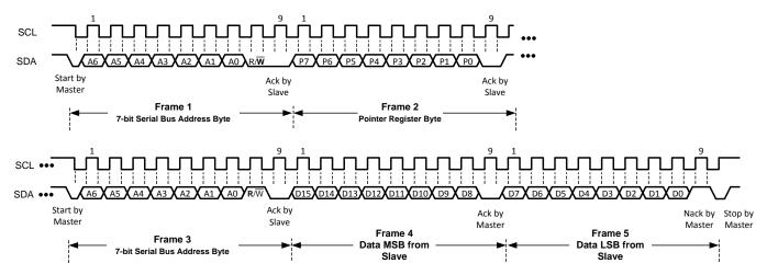
Figure 11. Reading Frame (Configuration Register)
