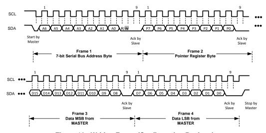
Figure 10. Writing Frame (Configuration Register)
