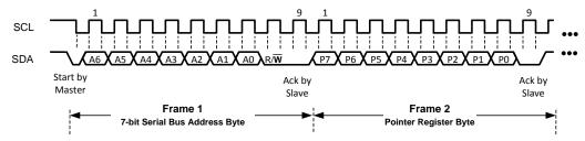
Figure 12. Trigger Humidity/Temperature Measurement
