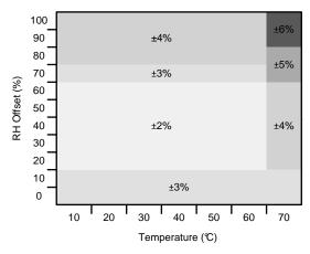
Figure 17. Relative Humidity Accuracy vs Temperature
