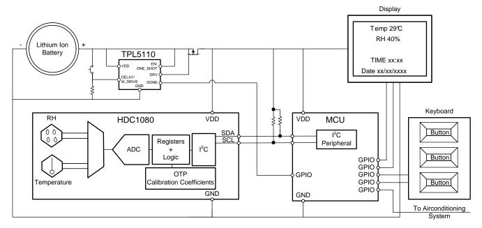
Figure 15. Typical Application Schematic HVAC
