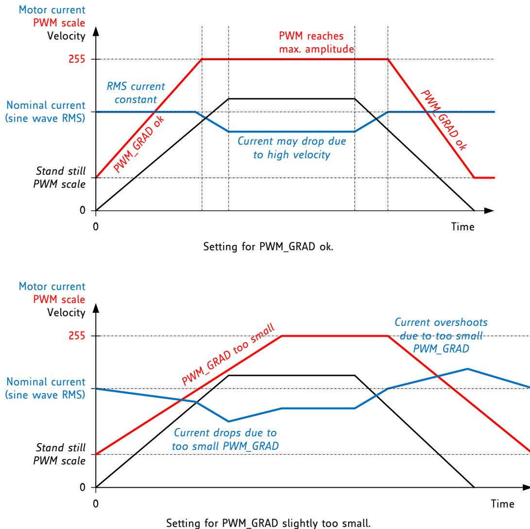
**Figure 6.4 Good and too small setting for PWM\_GRAD**
