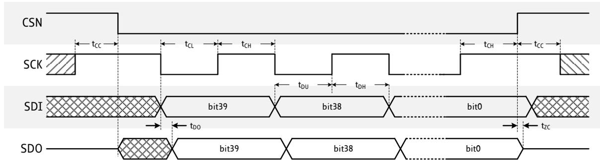
**Figure 4.1 SPI timing**
