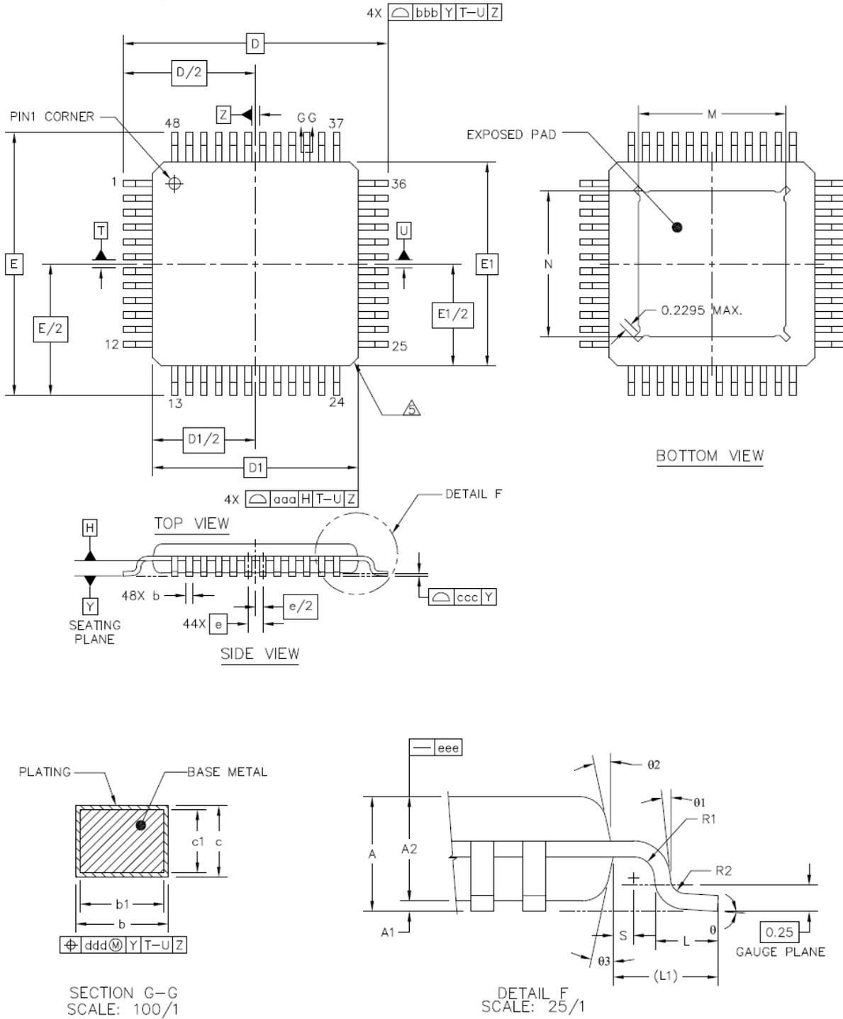
Figure 30.2 Dimensional drawings TQFP-EP48
