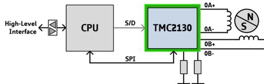
In this application, the CPU initializes the TMC2130 motor driver via SPI interface and controls motor movement by sending step and direction signals. A real time software realizes motion control.
