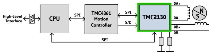
The CPU initializes the TMC4361 motion controller and the TMC2130. Thereafter, it sends target positions to the TMC4361. Now, the TMC4361 takes control over the TMC2130. Combining the TMC4361 and the TMC2130 offers diverse possibilities for demanding applications including servo drive features.
