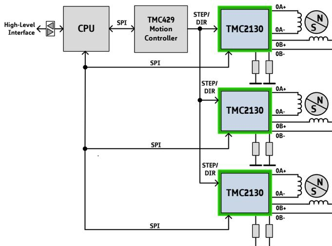
Here, an application with up to three stepper motors is shown. A single CPU combined with a TMC429 motion controller manages the whole stepper motor driver system. This design is highly economical and space saving if more than one stepper motor is needed.
