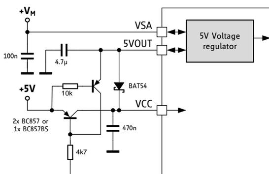
VCC supplied from external 5V using active switch. 5V or 3.3V IO voltage.
