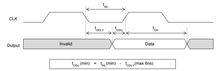
Figure 2 Output timing
