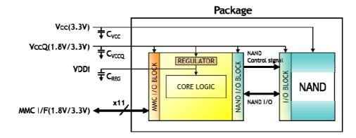
Figure 1 THGBMFG7C1LBAIL Block Diagram
