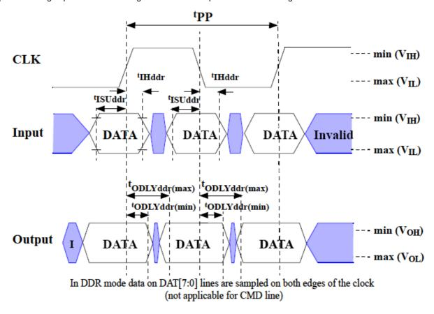
High-speed dual data rate interface timings
