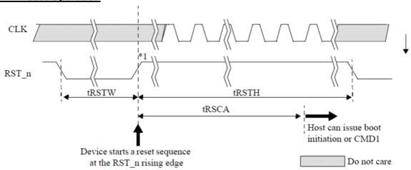
(Note) \*1 : Device will detect the rising edge of RST\_n signal to trigger internal reset sequence
