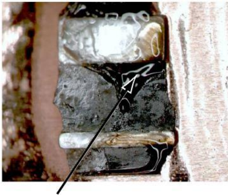
Figure 9 Flux residue compromising isolation
