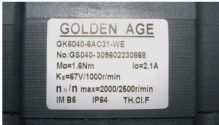
Figure 1—Motor Nameplate.
