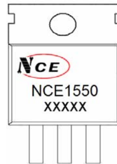
Marking and pin assignment
