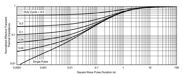
Normalized Thermal Transient Impedance, Junction-to-Ambient
