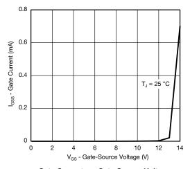
Gate Current vs. Gate-Source Voltage
