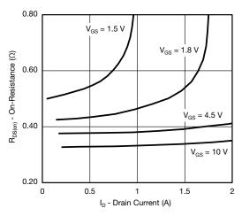
On-Resistance vs. Drain Current
