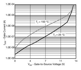
Gate Current vs. Gate-Source Voltage
