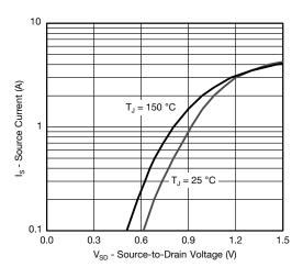
Soure-Drain Diode Forward Voltage
