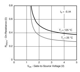
On-Resistance vs. Gate-to-Source Voltage
