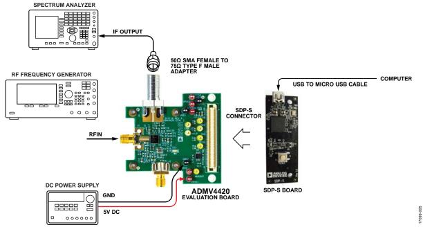
Figure 5. ADMV4420-EVALZ Lab Connections
