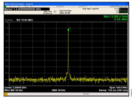
Figure 21. ADMV4420 Results with a 20.2 GHz LO, 18 GHz RF Signal at -40 dBm, and 50 MHz On-Board Crystal Oscillator
