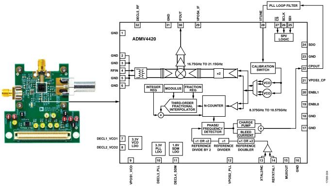
Figure 4. Evaluation Board Configuration
