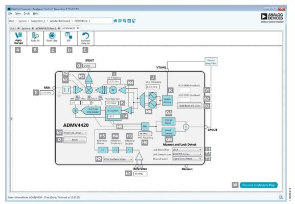
Figure 13. ADMV4420 Main Block Diagram with Labels
