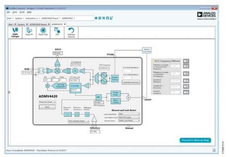
Figure 14. ADMV4420 Block Diagram Labels for VCO Locked Frequency vs. Requested Frequency Difference
