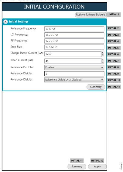
Figure 12. ADMV4420 INITIAL CONFIGURATION Menu with Labels
