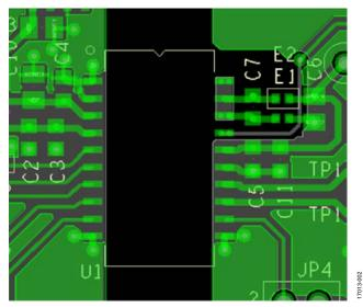
Figure 2. Layout Example for EVAL-ADM3055EEBZ
