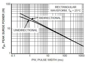
Figure 8. Maximum Non-repetitive Surge Power, P<sub>pk</sub> versus PW
