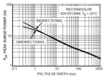
Figure 9. Maximum Non-repetitive Surge Power, Ppk(NOM) versus PW
