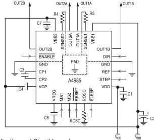
Figure 8: ES Package Typical Application and Circuit Layout
