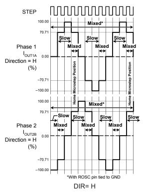
Figure 10: Decay Mode for Full-Step Increments
