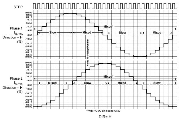
Figure 13: Decay Modes for Eighth-Step Increments
