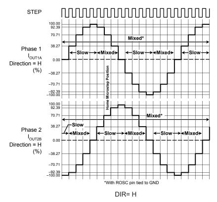
Figure 12: Decay Modes for Quarter-Step Increments
