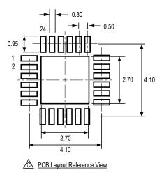
For Reference Only; not for tooling use (reference JEDEC MO-220WGGD) Dimensions in millimeters
