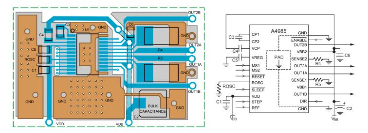
Figure 9: LP Package Typical Application and Circuit Layout
