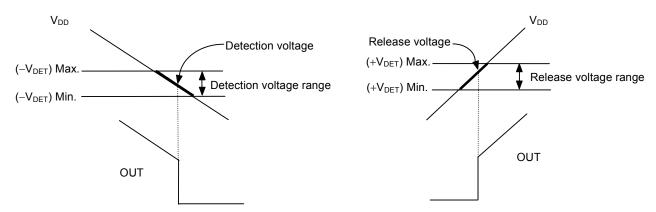
Figure 18 Detection voltage (CMOS output products)
