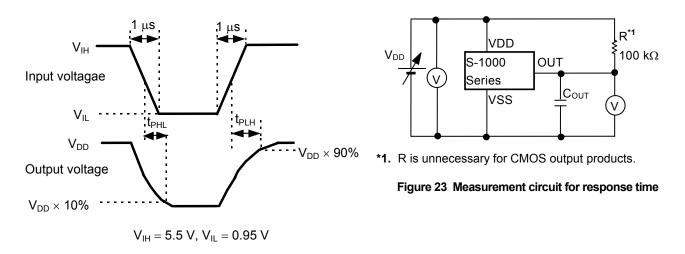
Figure 22 Measurement condition for response time
