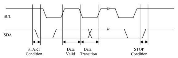
Figure 1: Timing diagram for START and STOP conditions
